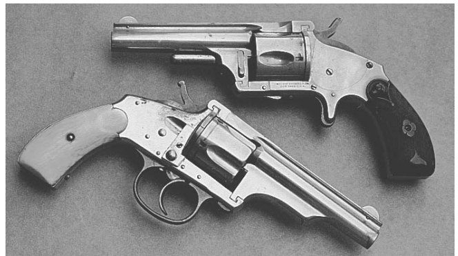
Top: Single-Action Pocket Revolver. Bottom: Double-Action Pocket Revolver Courtesy Supica's Old Town Station
