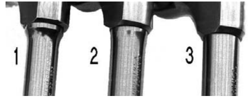
The three barrel profiles used with the Colt pre-Woodsman and First Series Target Model: from left to right, in order used, the pencil barrel, medium weight barrel, and straight taper barrel.
