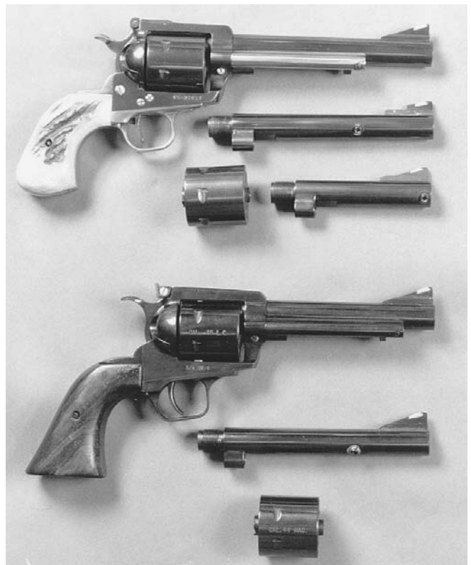
Two examples of Quik-Kit revolvers. At the top is a Ruger reworked by United Sporting Arms, Inc. of Tucson and at the bottom is a standard production revolver from the same company.
