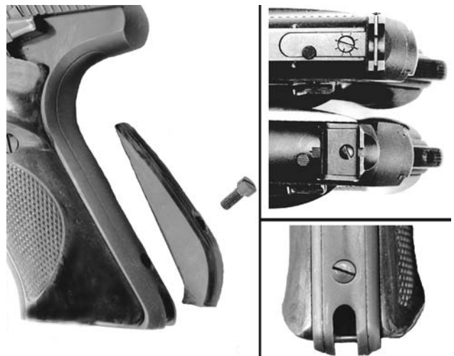
(Above left) The Second Series Woodsman came with two grip adapters, to provide for different sized hands.
