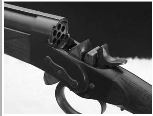
Closeup of the receiver of the Pieper Volley Gun. Note the general resemblance to the Remington Rolling Block
